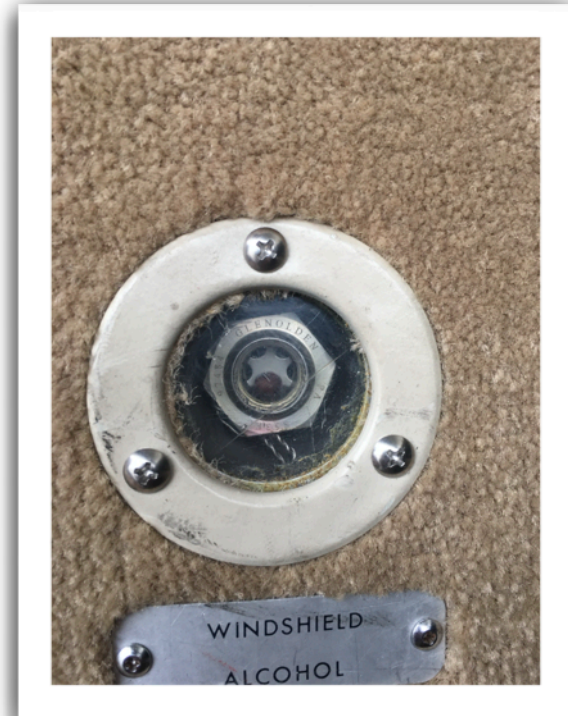
Example of empty alcohol tank during preflight
